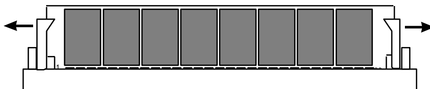
Figure 37 - Removing SIMMs
