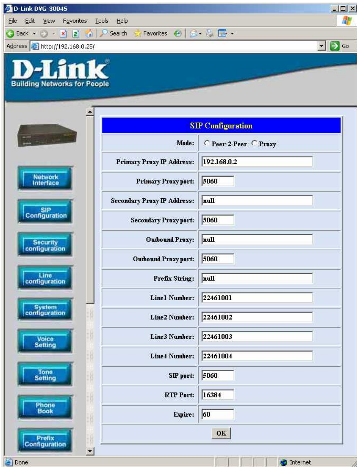
Screenshot 19 – D-Link DVG-3004S gateway SIP configuration
