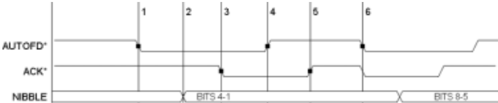
Figure 42: Nibble mode cycle
